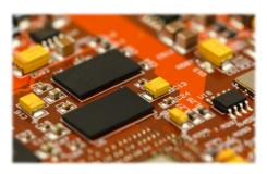
Tantalum capacitors (yellow) on an electrical circuit board (Shutterstock)
