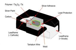
A typical chip tantalum capacitor (KEMET Electonics)
